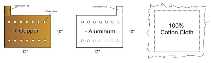
Figure #1 Top View of separate pieces
