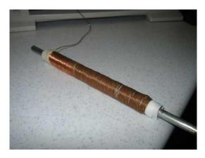
Our small test model #1, we used #22 bare copper wire wrapped around a zinc rod, each layer had a paper die electric, tested in tap water. 5 layers. Output = 89 vdc x 3.5 ma, this is low. more layers will = more capacitance which ='s more amperage and voltage.
