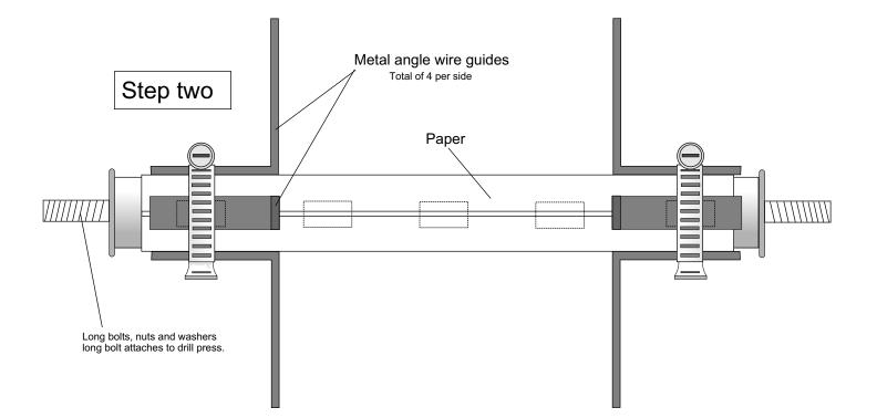
Apply first layer of wire, remove, metal wire guides, apply more paper, then repeat over and over again until you have about a 5 to 6 inch diameter roll of wire and paper. Makes a very powerful earth capacitor!
